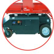
Wide drive and steer wheels–for reduced ground pressure and increased traction on tough job sites.
