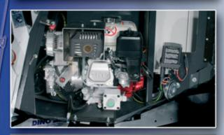
Petrol or diesel power pack is standard - power for lift also without mains.
